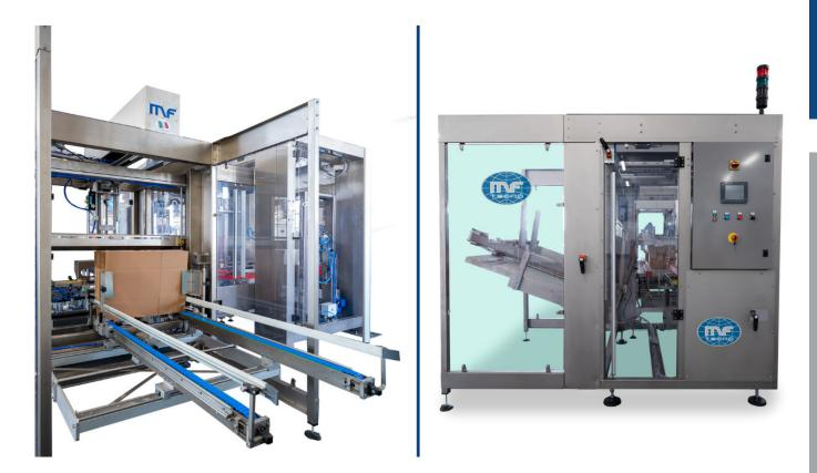
The closed cardboard is picked up from the dispenser and opened by means of suction cups mounted on a mechanical arm.
