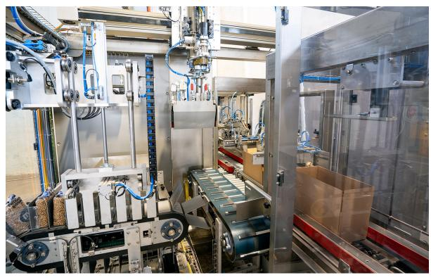
The flaps opening system can be either automatic or semi-automatic. This system guarantees the perfect centering of the box at the time of insertion by Pick and Place. After the filling station, the American case (RSC) is transported to the upper closing station. The sealing can take place by means of tape, hot melt or with both methods.
